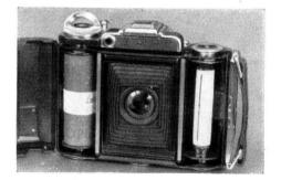
4. Draw the spring stud (19) outwards and take out the spool. It is advisable to protect it from the light by keeping it in the light-tight tin foil in which it was originally packed.
