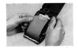
4. By giving a few turns to the winding key (12) in the direction of the arrow, draw the paper taut. While doing this, see that the paper is wound on straight. Any crookedness of the paper band should be put right before proceeding further.
