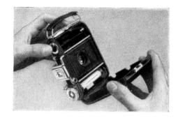
2. Place the full spool in the feed chamber (18) while drawing the spring stud outwards. The tapered end of the paper leader must point towards the take-up spool chamber (19), which contains an empty spool on which the exposed film is wound.
