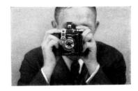
The camera may also be held by gripping the front with the right hand and operating the milled disc (4) with the thumb. But in this case, the thumb must not be allowed to slow down the shutter lever as it fires.
