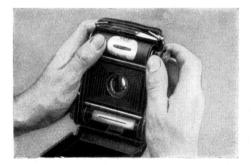
3. Detach the gummed strip which holds the protecting paper in place, and insert the end of the latter in the wide slit of the empty spool. In this position the black side of the paper should face downwards.
