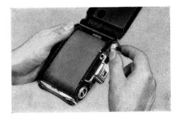
One half of the outer ring on the film winding key (12) is hinged and when lifted in the manner shown in the illustration opposite, affords a convenient grip for winding on the film.
