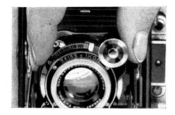
When setting the shutter, and this applies particularly to the speeds of  $^{1}/_{250}$  and  $^{1}/_{500}$  sec. a rather considerable resistance has to be overcome. To avoid overstraining the shutter mechanism or damaging the front carrying the lens, a counter pressure must be exercised when setting the shutter, as shown in the lower illustration on page 18.
