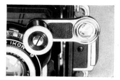
Observation is made in the viewing aperture (17). A circular light coloured field will be seen, in which all objects appear with double outlines.
