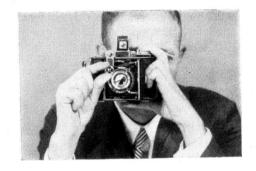
As the setting disc (3) is turned, these double images gradually coincide. When this is the case, the distance meter and the lens are accurately focussed on the object.
