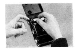
6. Turn the winding key (12) until it snaps with a click into the spool and turn the spool with it.
